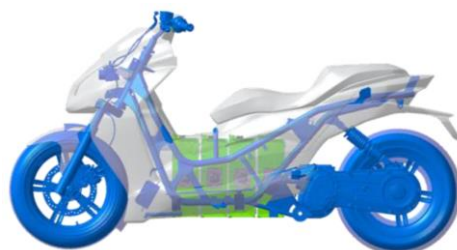
Figure 2 : Example of L3e vehicle with 4 battery modules shown in green
